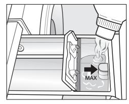
■ Add the fabric conditioner or liquid starch to the ⊗ compartment or insert the appropriate capsule. **Do not exceed the maximum level mark.**
